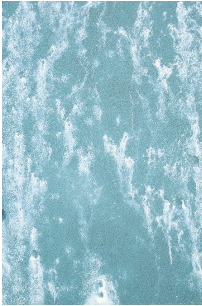
Figure 10 — Degree of rusting WRi 5
