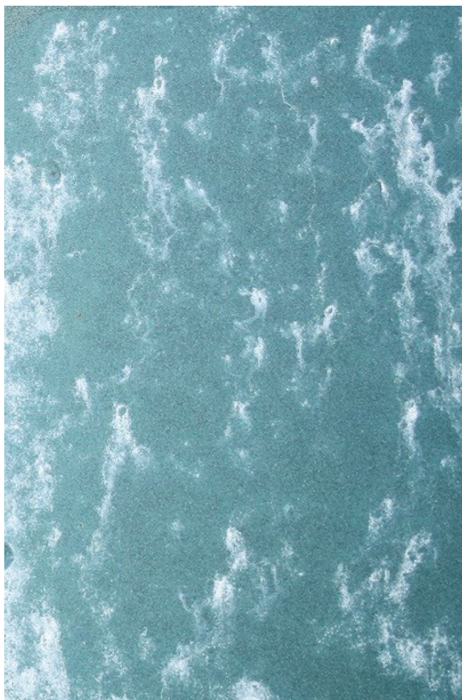
Figure 9 — Degree of rusting WRi 4
