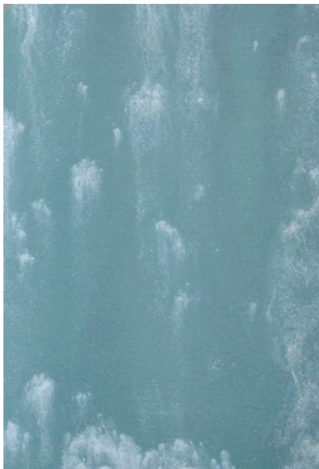
Figure 7 — Degree of rusting WRi 2
